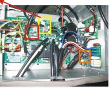
VP2--Intelligent Power Module / Power Source Board
