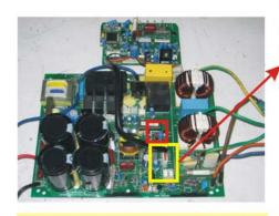
VP1--Intelligent Power Module /Power Source Board
